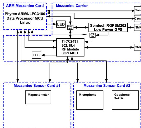
Fig. 3. Proposed modular node architecture
