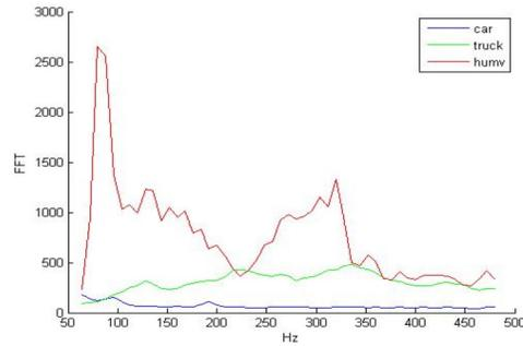
Fig. 1. Mean FFT coefficients for 3 vehicle classes
